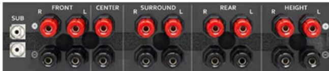
Figure 2: Rear panel of AVR; the height speaker connections are at right.
